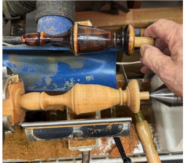
Turning a replacement bedpost finial for 12 yr old granddaughter of church friend.
